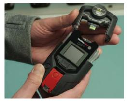
G7 features the industry's first expandable interface that enables customization to support each customer scenario and requirement. G7 functionality expands using one of four field-replaceable cartridges—a Standard Cartridge, Single-gas Diffusion Cartridge, a Multi-gas Diffusion Cartridge and a Multi-gas Pump Cartridge.
