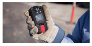
Blackline's G7 product line supports lone worker monitoring applications with or without the requirement for gas detection. For dedicated lone worker monitoring, G7 devices are fitted with a Standard Cartridge rather than a gas sensor cartridge. Safety monitoring options offered by G7 devices for lone worker includes True Fall Detection®, no-motion (mandown) detection, missed employee check-in, SOS latch and a silent SOS button.
