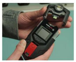
G7 features the industry's first expandable interface that enables customization to support each customer scenario and requirement. G7 functionality expands using one of four field-replaceable cartridges—a Standard Cartridge, Single-gas Diffusion Cartridge, a Multi-gas Diffusion Cartridge or a Multi-gas Pump Cartridge.
