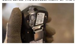
Blackline's in-house hardware and firmware teams completed the development work required and submitted the final G7 pump cartridge for intrinsic safety certification. This new cartridge expands beyond previous diffusion-based cartridges, enabling users to remotely sample the atmosphere of a tank, sewer or other confined space in order to understand whether potential gas hazards are present. The internal pump draws air samples from the remote location through up to 100 feet of tubing.
