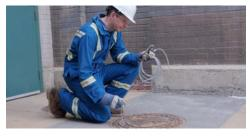
Blackline began delivering its certified G7 pump cartridge and shipped the first 1,000 units from its orders backlog. This new cartridge enables G7 safety wearables to be equipped with the functionality needed to support confined space entry and leak check scenarios. Air is remotely sampled through a length of tubing, or using a probe, to determine whether any gas-based hazards exist in a confined space or are leaking from equipment or piping.
