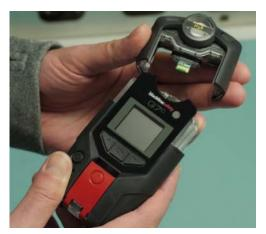
G7 wearables feature the industry's first expandable interface that enables customization to support each customer scenario and requirement. G7 functionality expands using one of four field-replaceable cartridges—a Standard Cartridge, Single-gas Diffusion Cartridge, a Multi-gas Diffusion Cartridge or a Multi-gas Pump Cartridge.
