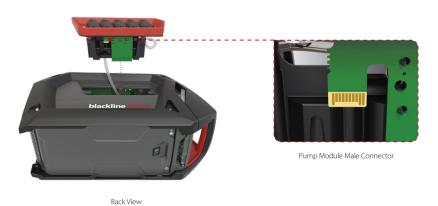
Figure 4-4: Location of G7 EXO pump module male connector
