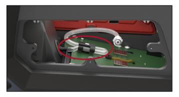
Figure 4-7: Ideal tubing position for optimal gas flow
