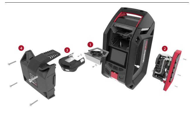
Figure 4-1: Installing G7 EXO Pump components
