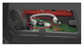
Figure 3-5: Ideal tubing position for optimal gas flow
