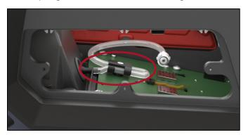
Figure 3-2: Ideal tubing position for optimal gas flow
