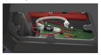
Figure 4-2: Ideal tubing position for optimal gas flow
