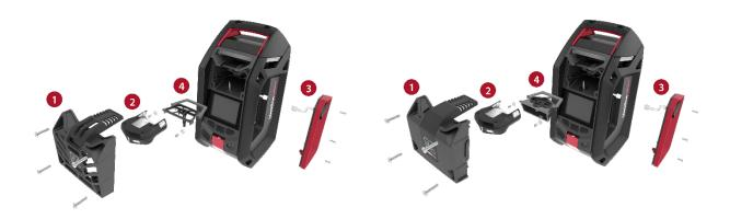
Figure 3-3: Uninstalling updated G7 EXO Diffusion components
