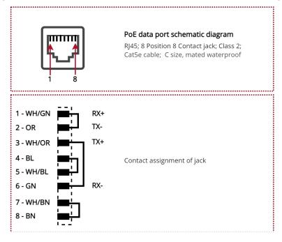
G7 EXO Translator PoE data port aligns with the standard IEEE802.3af, power class 2 parameters:
