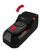
3. Close G7 Dock's lid and press down firmly until the release tabs click into place on both sides.
