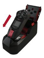
1. Slide G7 device into G7 Dock's charge clip at an angle. Ensure the charge clips of both devices are connected.
