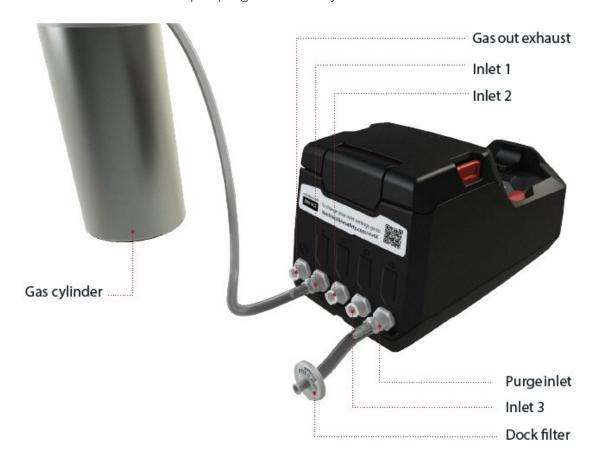
When looking at the back of G7 Dock, the Gas out exhaust is the connector on the far-left side of the dock. It is used to transfer calibration gas to a safe exhaust location.
