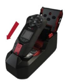
2. Keeping the charge clips connected, lie G7 down into G7 Dock and push down until the device clicks in place.
