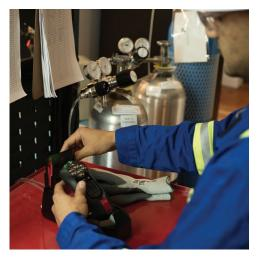
G7 Dock is Blackline's solution to gas sensor calibrating, bump testing and charging G7. It supports both G7c and G7x devices with single-gas, multi-gas diffusion or multi-gas pumped cartridges.
