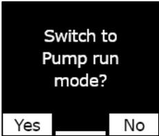
**NOTE:** If the mode selected uses a pump, G7 will test the pump flow before entering the mode.
