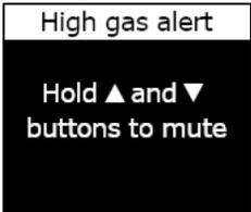
**NOTE:** A device equipped with an O<sub>2</sub> sensor will activate high gas notifications in both oxygen-deficient and oxygen-enriched environments.
