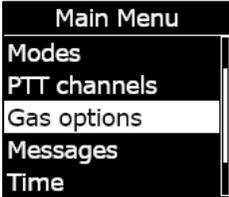
3. Using the up and down arrow buttons, scroll through the menu and select **Gas Options** by pressing the OK button. The Gas info menu opens.
