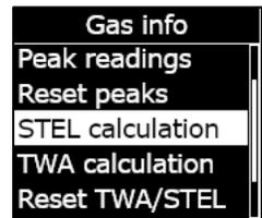
By default, the STEL value for your device automatically resets when your device is power cycled. You can manually reset the STEL value for your devices using the Gas info menu.
