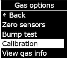
4. Using the up and down arrow buttons, scroll through the menu and select **Calibration** by pressing the OK button.
