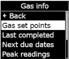
The Gas set points screen opens, displaying the gas sensor set points for your device.
