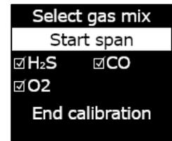
8. Use the up and down arrow buttons to select **Start span** and press the OK button to start the calibration.
