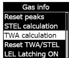
By default, the TWA value for your device automatically resets when your device is power cycled. You can manually reset the TWA value for your devices using the Gas info menu.
