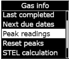
By default, the peak gas readings for your device automatically reset when your device is power cycled. You can manually reset peak gas readings for your devices using the Gas info menu.
