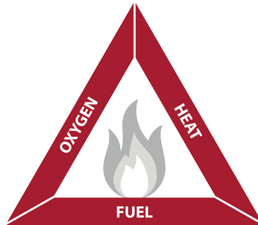
Figure 1: The fire triangle, which identifies the three necessary elements for a fire to burn.
